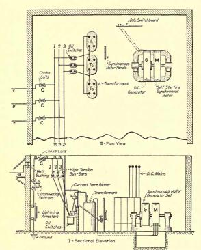
Fig. 142.—Typical arrangement of a synchronous motor-generator substation.
